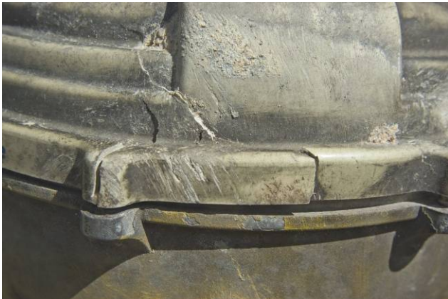
Figure 7: Damage from 4m drop onto blade. Radome repair was fast and inexpensive
