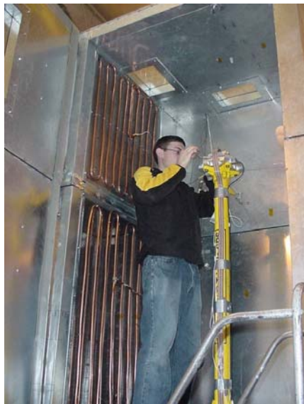
Figure 3: Trimble MS980 and installation mast on the shake table with temperature cycling tubes in the background
