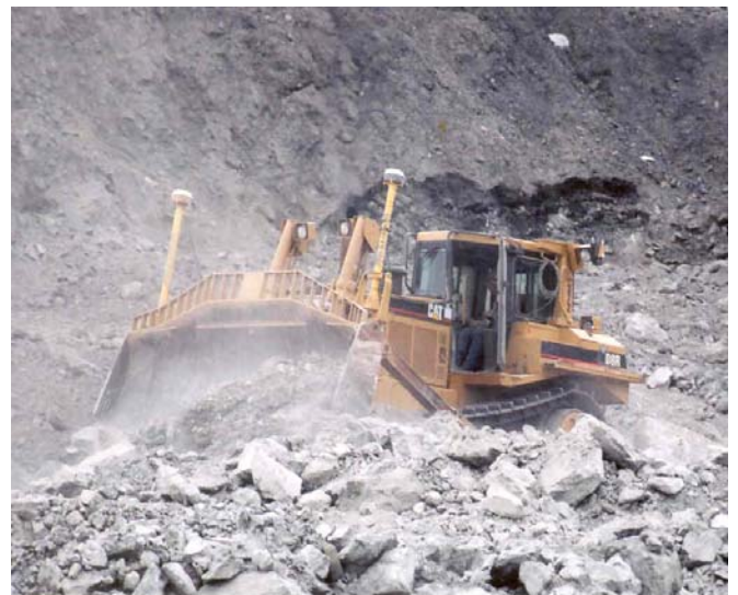
Figure 4: Field testing on hard rock pushed the Trimble MS980s past their expected operating conditions. High-accuracy RTK was maintained under these conditions.
